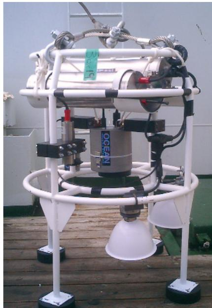
Camera system mounted on a frame for bottom contact (pogo) operation.
