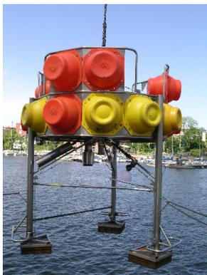
Camera mounted on a tripod for long term deployment.
