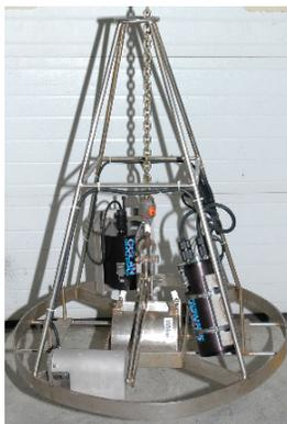
Camera system mounted on a bottom grab.
